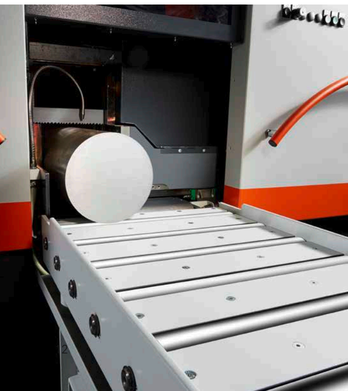
Infeed and outfeed roller conveyors with different lengths and versions
