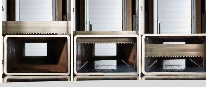
The system controls the cutting force continuously, so that the system is constantly at the permitted cutting force and does not exceed it. The saw downfeed optimises itself without intervention from the operator when this takes place. It leads to optimal productivity and also extends blade life.
