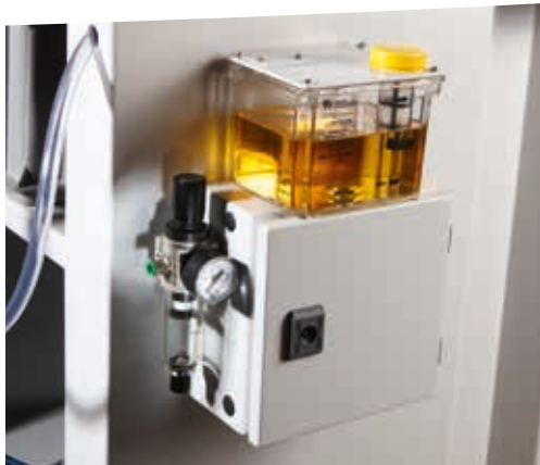
Micro-spray lubrication system.
