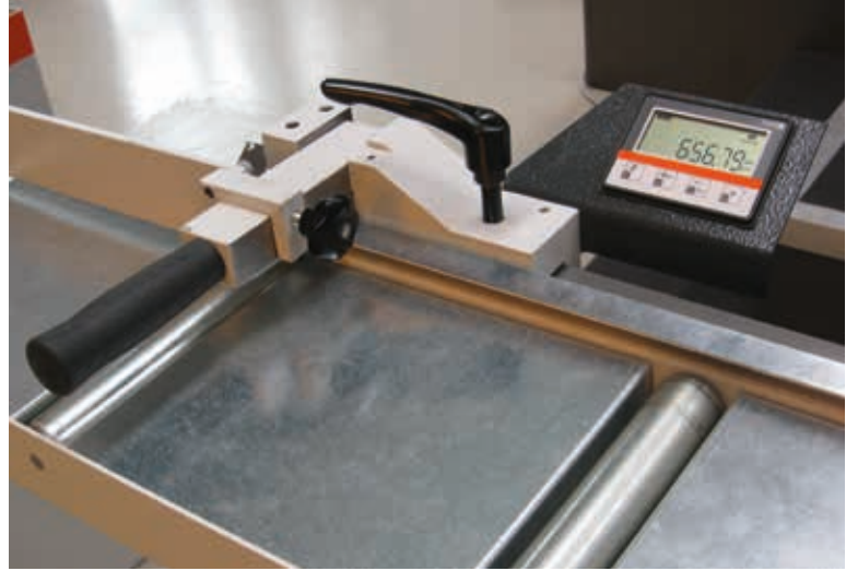
Digital measuring stop KASTOexact D 150.
