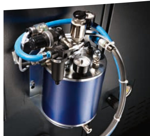
Micro-spray lubrication system.
