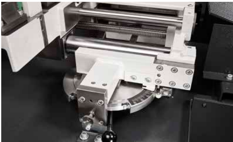
Material feed via ball screw spindle, infinitely adjustable mitre angle.
